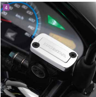
4 Silver Master Cylinder Cap This silver anodised aluminium version replaces the standard one for a more premium look.
